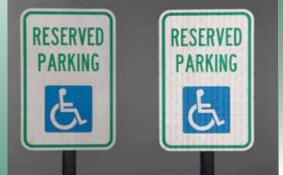
Engineer grade prismatic (right) microprismatic optics provides better daytime and nighttime brightness compared to beaded engineer grade (left).
